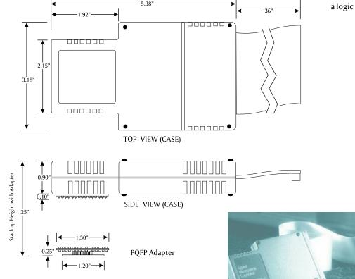
Probe Tip dimensions of the EL 3200 Emulator for Motorola 68330/340.
